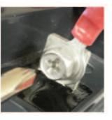
9) The Universal T-Adapter Connector is now securely fixed to the battery. You can fit a T-Adapter to use with your battery.
